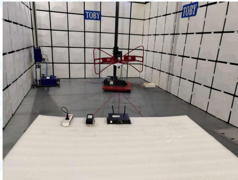
**Photo of Setup for Conducted Emission**
