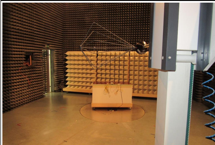
Test setup radiated below 0.2GHz
