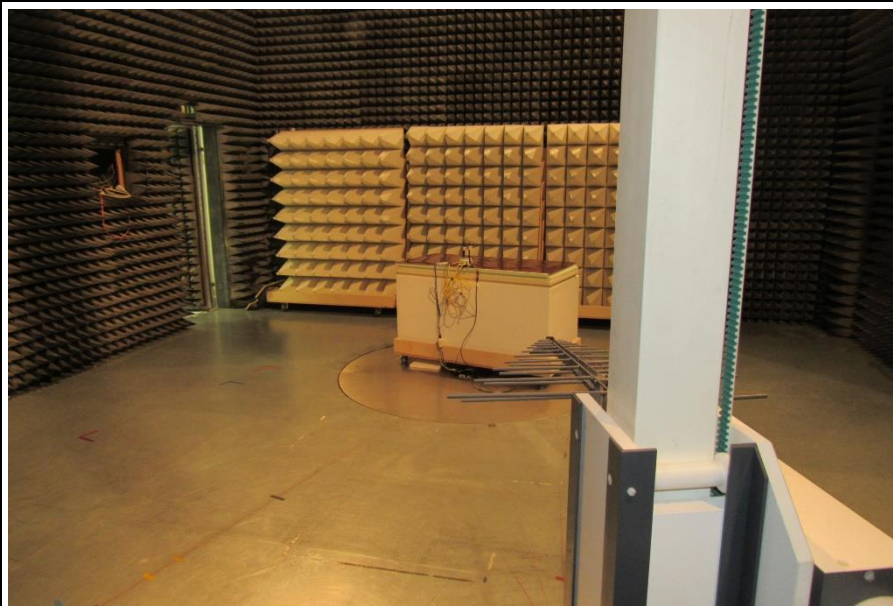
Test setup radiated between 0.2 to 1 GHz
