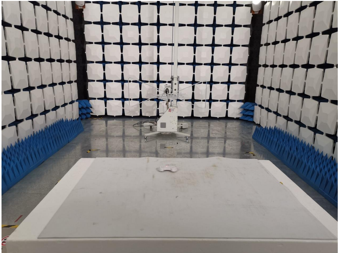
Below 1GHz for radiated emission test setup
