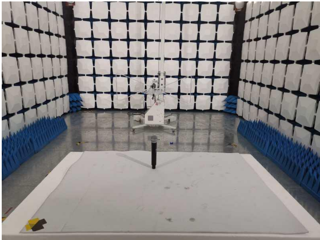
Below 1GHz for radiated emission test setup
