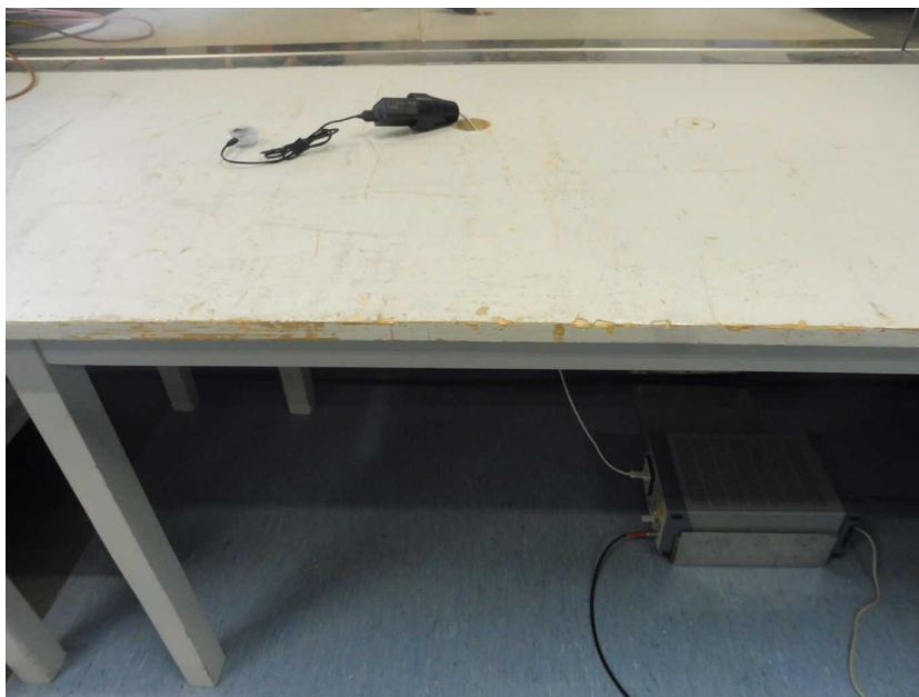
Photo 8: AC conducted emission test setup
