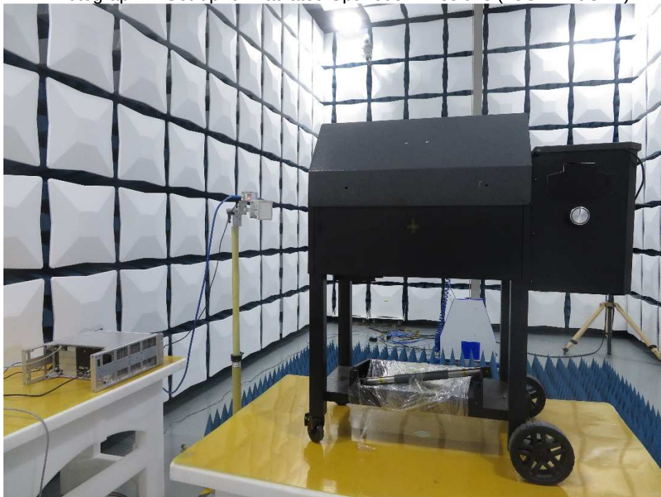
Photograph 2: Set-up for Radiated Spurious Emissions (18GHz-25GHz)
