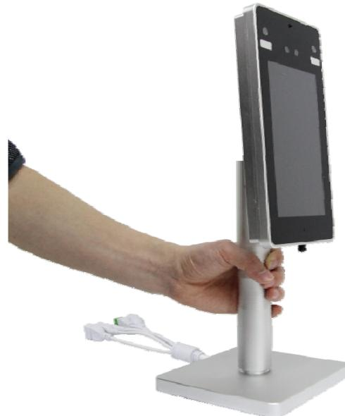
2.3. Connect the Ethernet and Power Cable to the Stand Base connectors.
