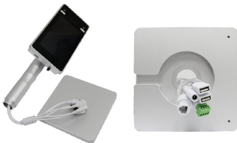
2.2. Screw the V3 mount into the base stand and secure it from the bottom using the helix nut provided. The mount is meant to be screwed in, not forced in directly.
