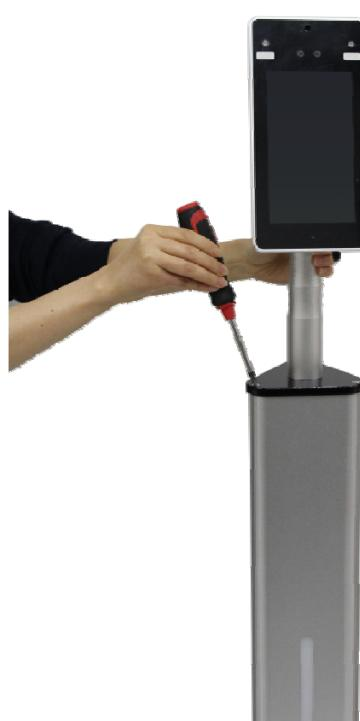
3.7 Upon completing installation, adjust the screen to the side with the blue light bar.
