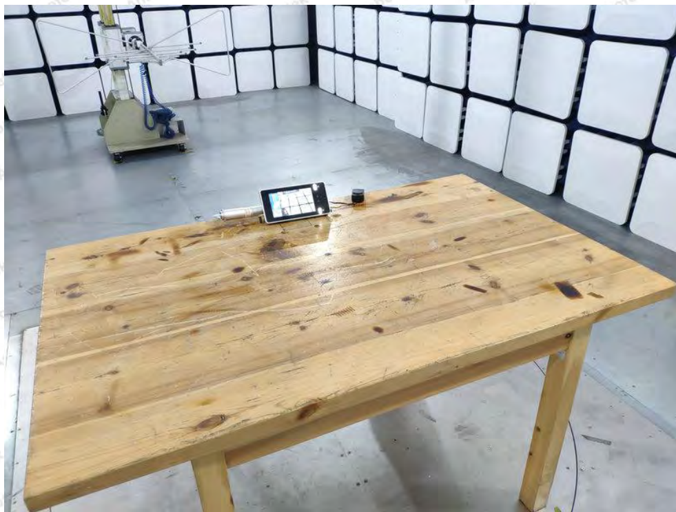
Photo of Radiation Emission Test
