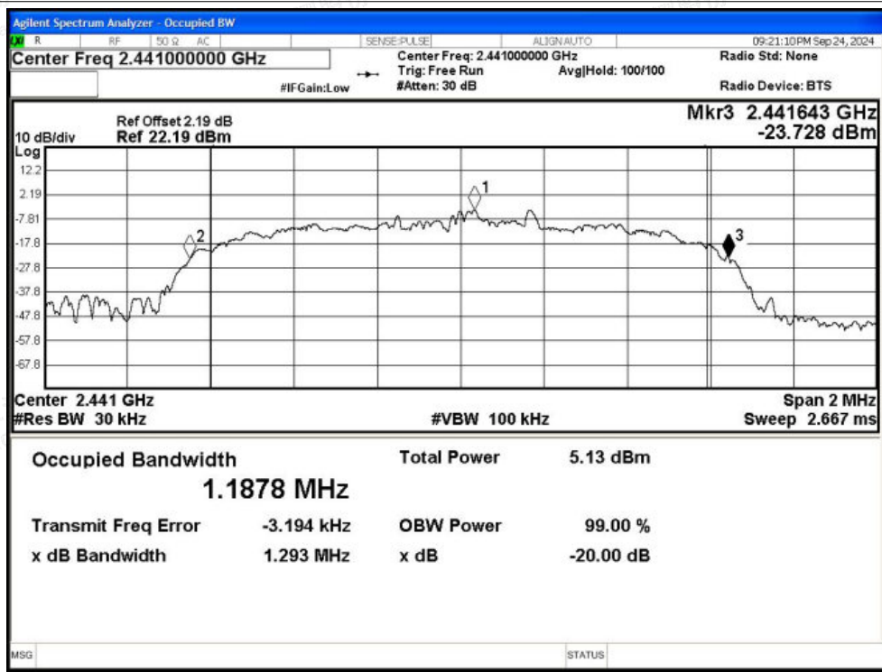
-20dB Bandwidth NVNT 3-DH5 2441MHz Ant1
