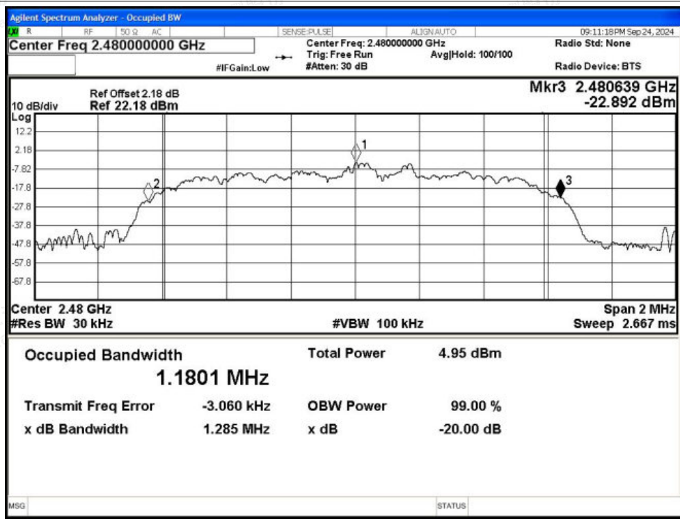
-20dB Bandwidth NVNT 2-DH5 2480MHz Ant1
