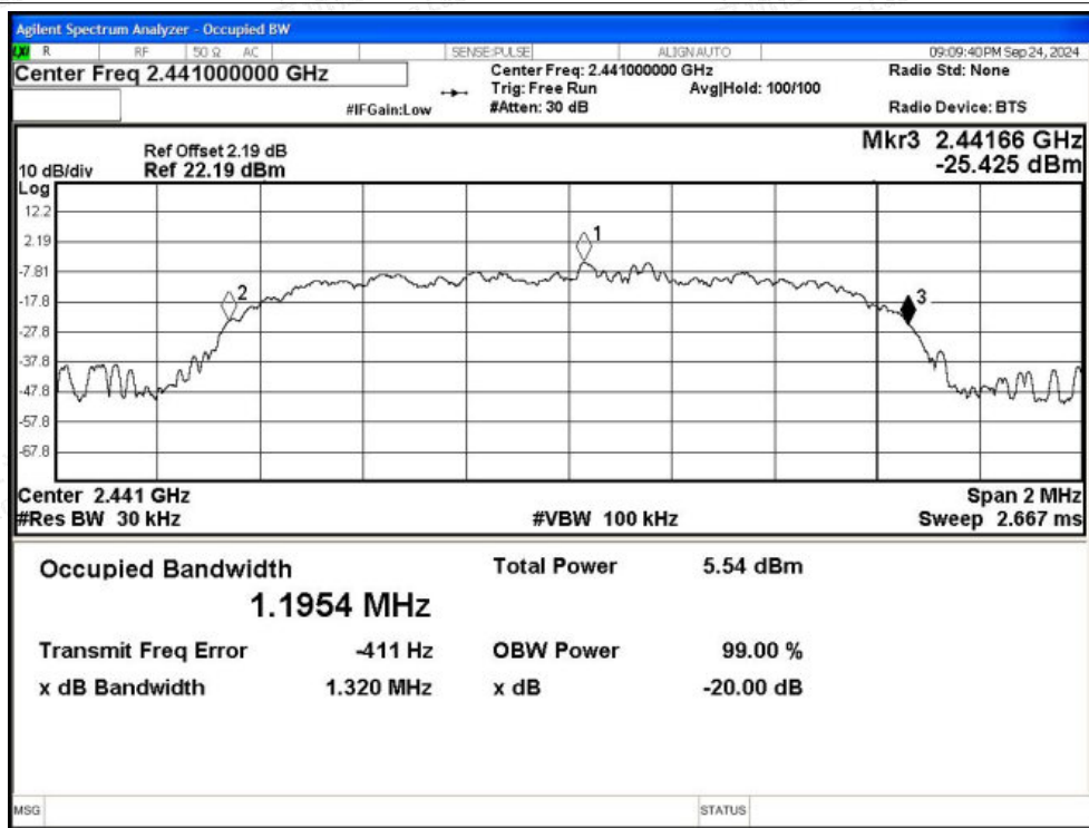
-20dB Bandwidth NVNT 2-DH5 2480MHz Ant1
