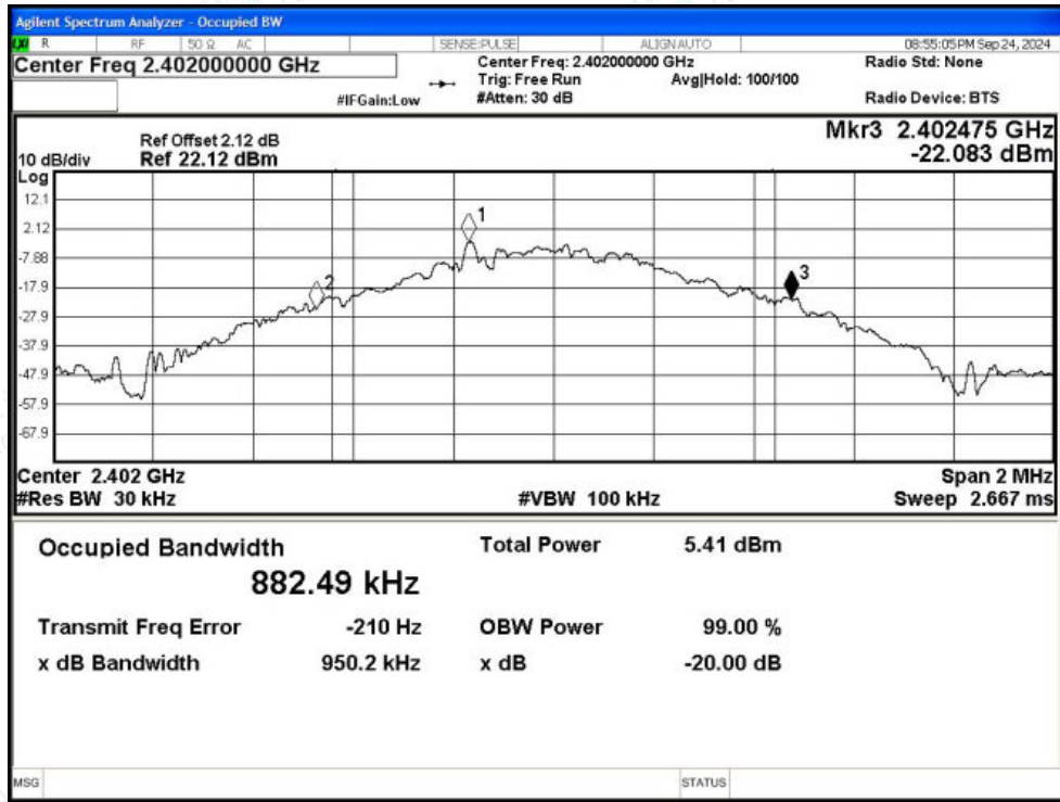
-20dB Bandwidth NVNT 1-DH5 2441MHz Ant1
