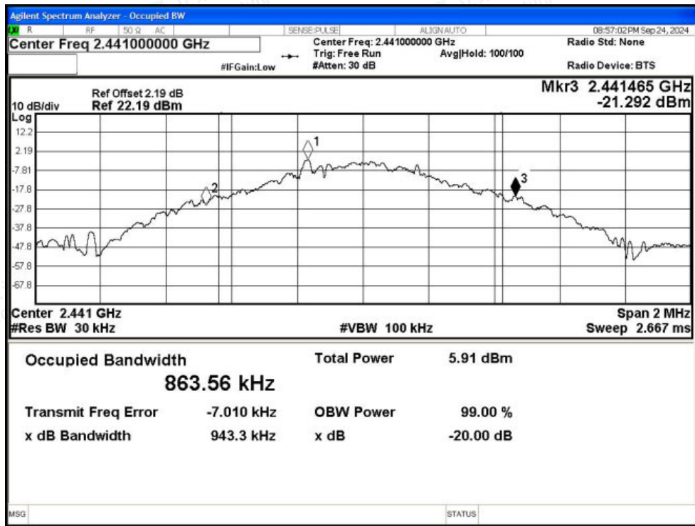
-20dB Bandwidth NVNT 1-DH5 2441MHz Ant1
