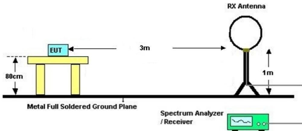
For radiated emissions from 30MHz to 1GHz
