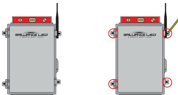
4. Use a 1/4" drill bit for the pilot holes. Use the Mounting Anchors and Screws provided to mount the Sector Selector to the surface.
