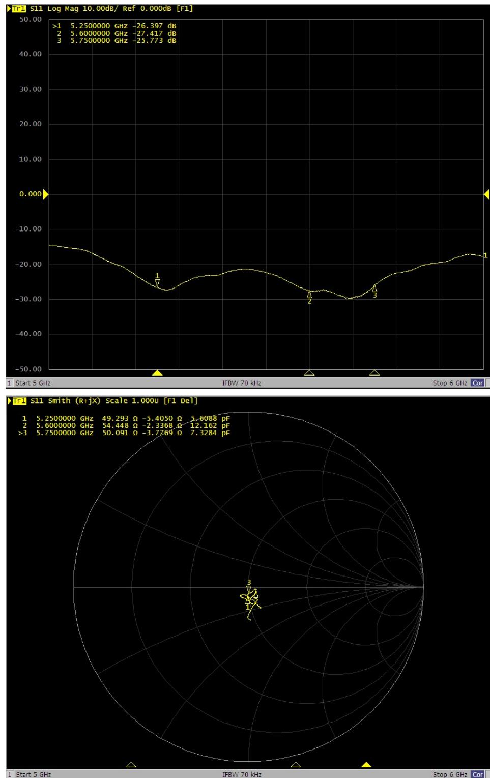
**<Dipole Verification Data> - D5000 V2, serial no. 1128 (Data of Measurement : 12.14.2021)**
