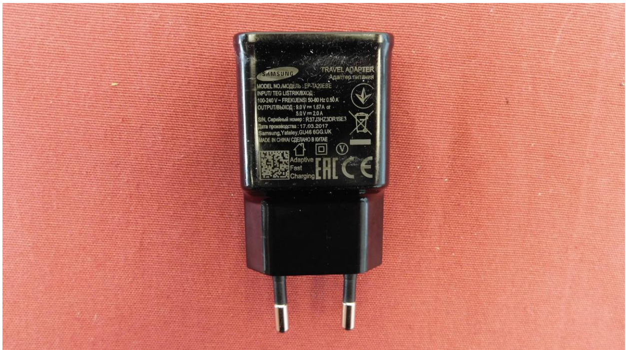
Picture 14: Power supply (only for AC powerline conducted emissions)
