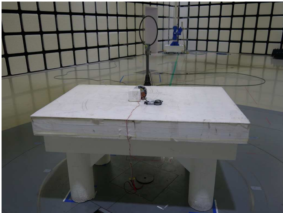
Photograph 2: Set-up for Radiated Spurious Emission below 30MHz, Rear View
