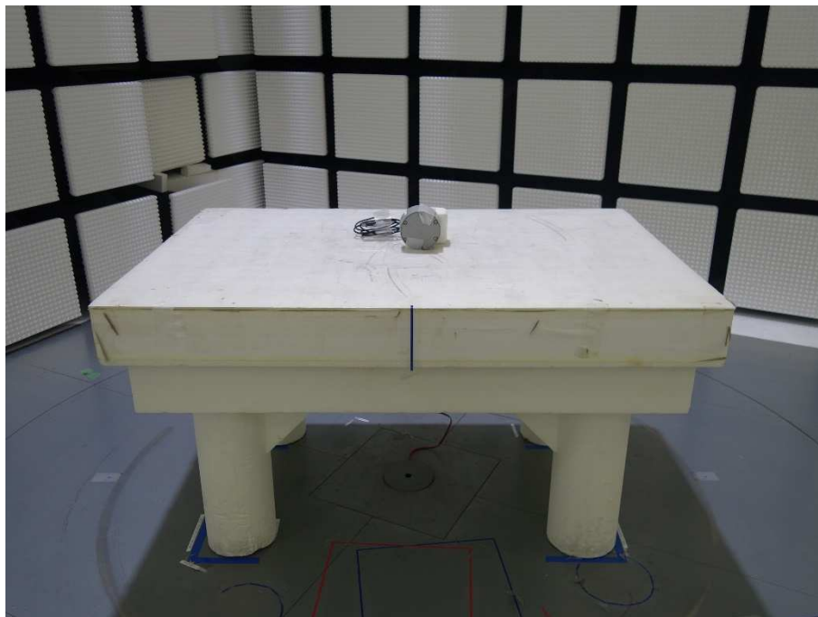
Photograph 3: Set-up for Radiated Spurious Emission below 1GHz, Front View
