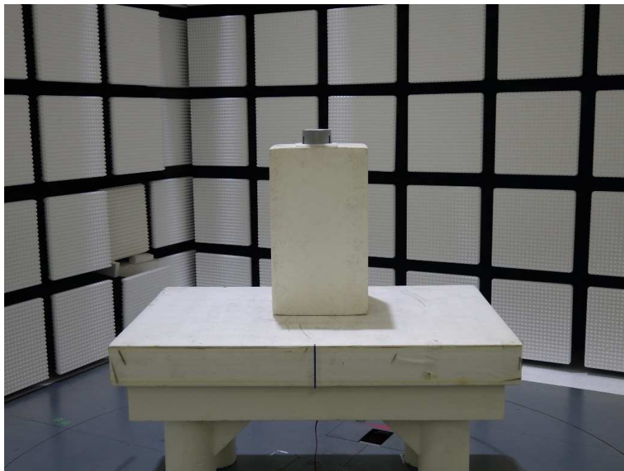
Photograph 7: Set-up for Radiated Spurious Emission above 1GHz, Front View
