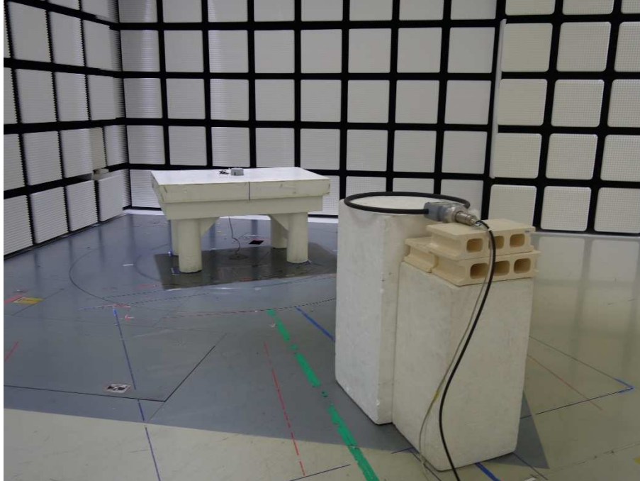
Photograph 3: Set-up for Radiated Spurious Emission below 30MHz, Front View
