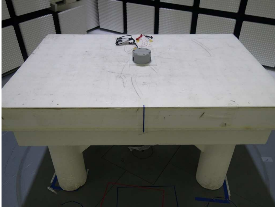
Photograph 5: Set-up for Radiated Spurious Emission below 1GHz, Front View
