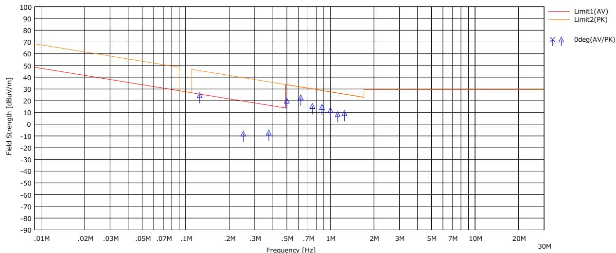
\* Data above 490 kHz were measured using a QP detector.
