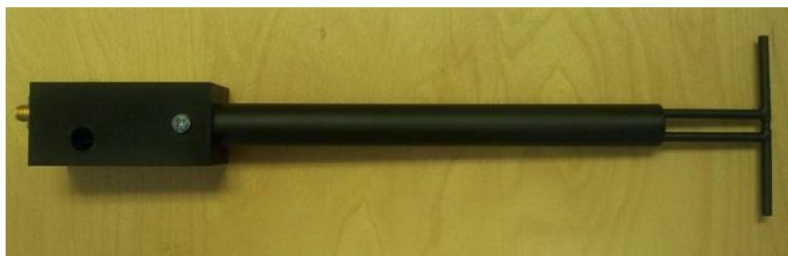
Figure 1 – MVG COMOSAR Validation Dipole
