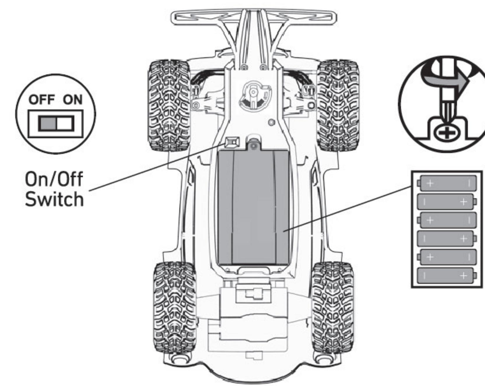
3 Open battery cover and install 1 9V battery (included). Replace the cover.
