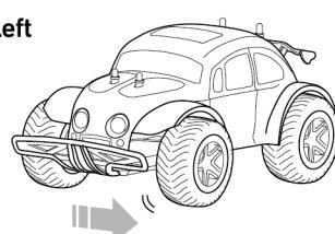
If the car tends to drift to the left, move the trimmer (beneath the car) to the left to adjust the steering.
