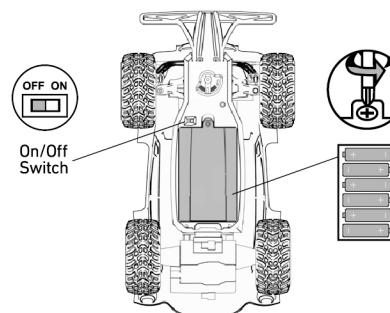
3 Open battery cover and install 1 9V battery (included). Replace the cover.
