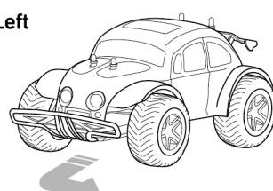
Push the throttle lever forwards and press the steering lever to the left.
