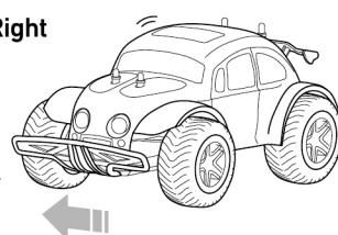
If the car tends to drift to the right, move the trimmer (beneath the car) to the right to adjust the steering.
