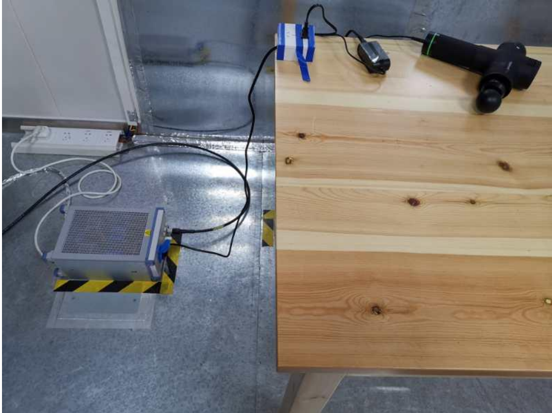
Power line conducted emission test setup
