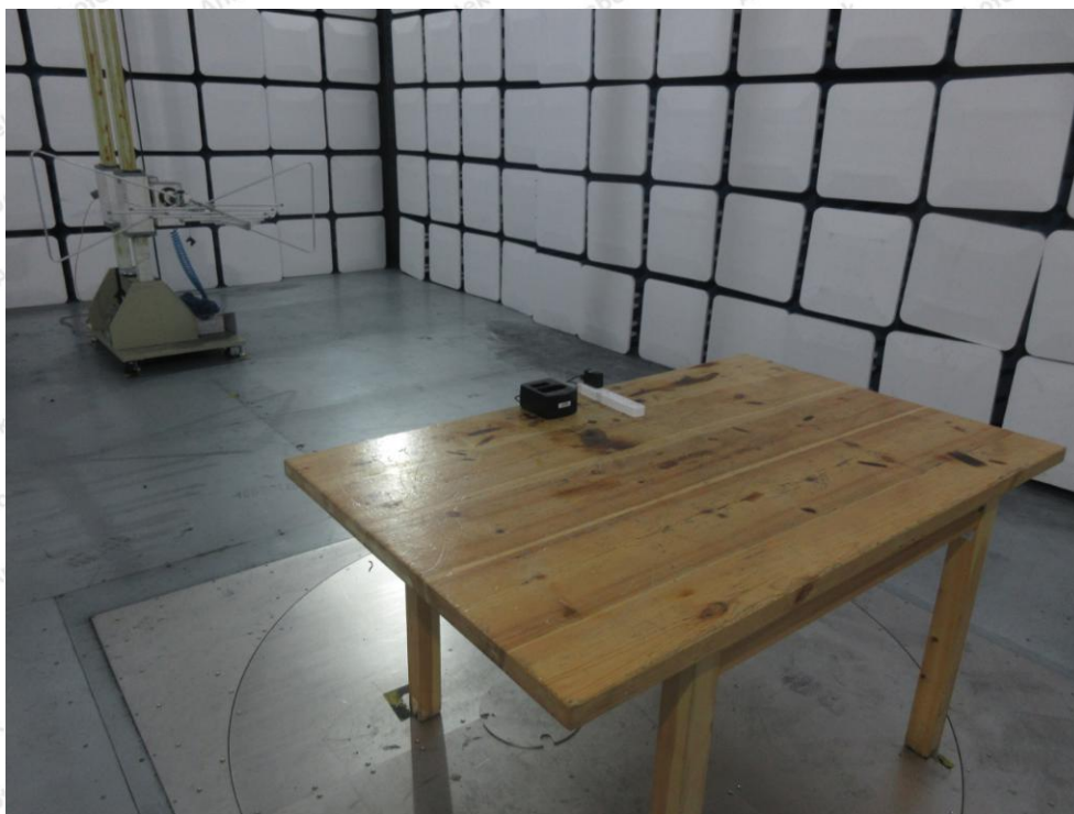
Photo of Radiation Emission Test
