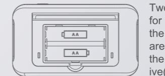
Two AA size Batteries are needed for F7 device. Place the batteries into the Battery Box and make sure they are put in the correct way by matching the positive(+) and the negative(-) pole.
