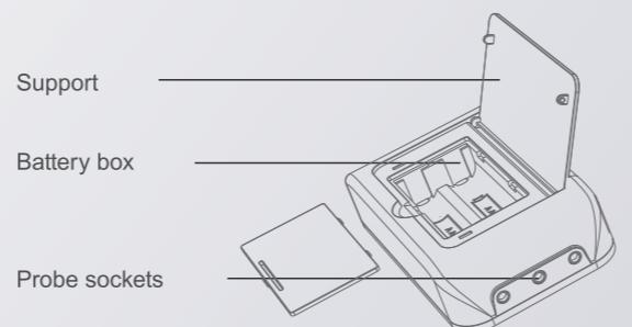
The device provides 6 sockets for the probes, which enable you to monitor up to six items simultaneously. Only two probes are included in the package. If you require more probes, please contact the dealer.
