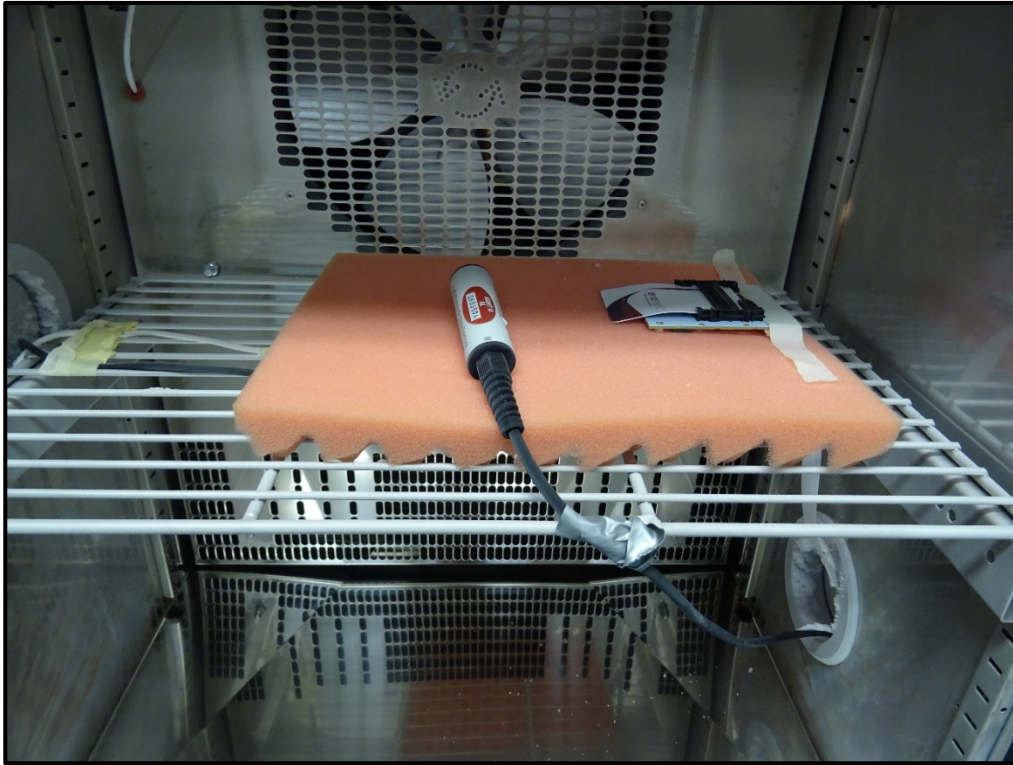
Photo 9 Frequency Stability (Temperature & Voltage Variation) Test Setup
