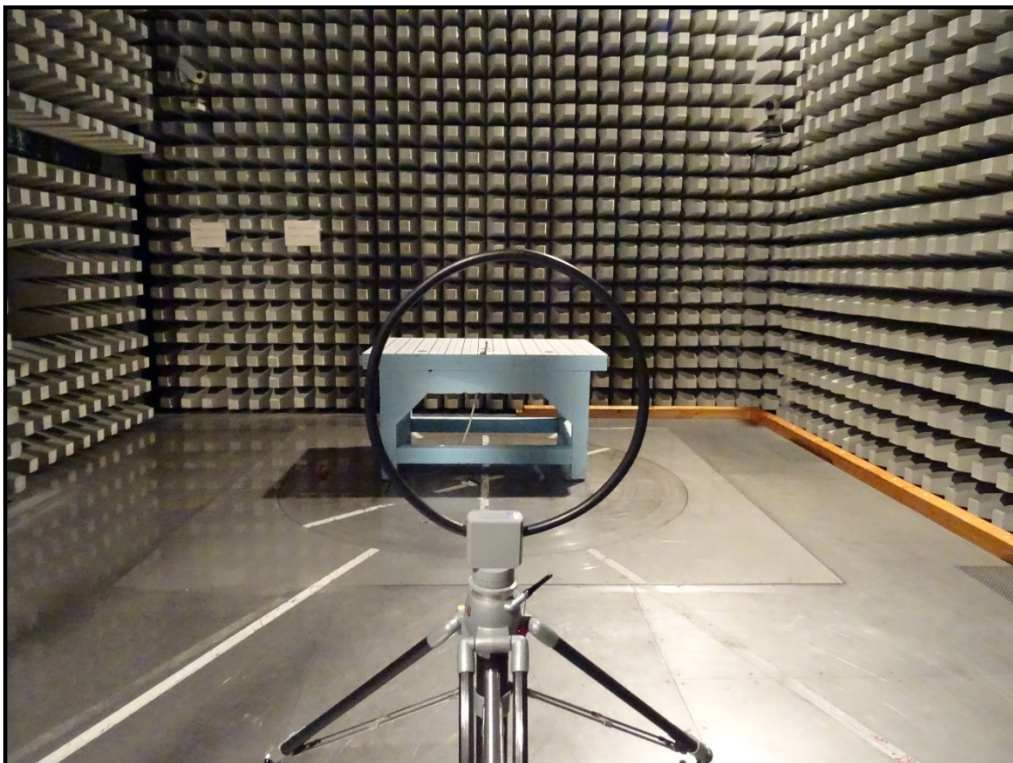
Photo 2 Radiated Test Setup-9 kHz – 30 MHz
