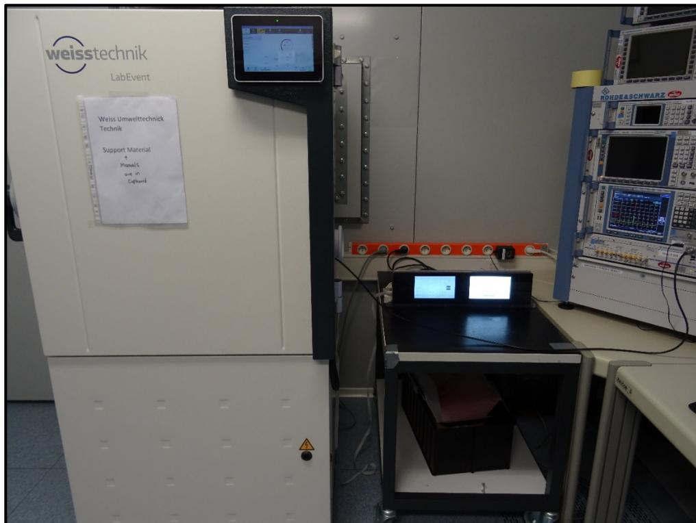
Photo 10 Frequency Stability (Temperature & Voltage Variation) Test Setup
