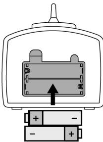
Replace the battery cover on controller in the direction as shown in .
