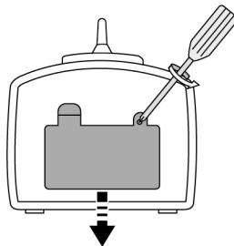
Set 2X1.5V battery in the correct direction.
