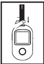
① With meter off or in setting mode and memory mode, insert a test strip to enter into testing mode.
