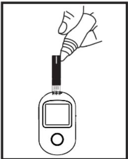
⑤ Touch and hold the hanging drop of control solution where the narrow channel meets the TOP EDGE of the test strip. Make sure the confirmation window fills completely. Control solution should not be applied to the flat face of the test strip.
