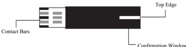
Contact Bar: Insert it into strip port. Push it all the way until it will go no further.
