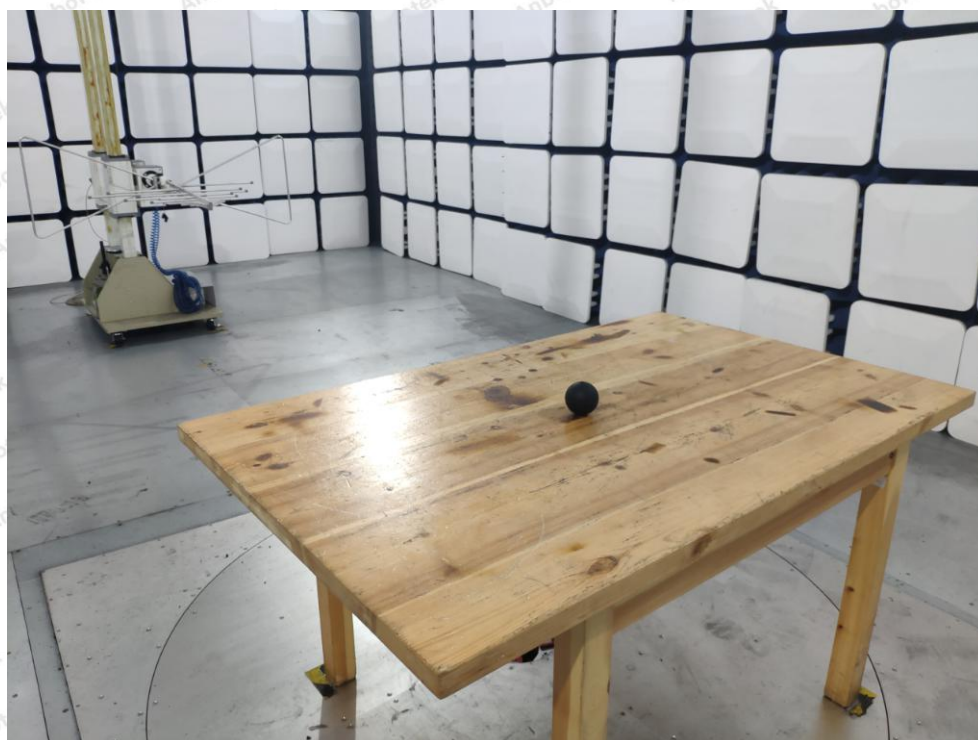
Photo of Radiation Emission Test
