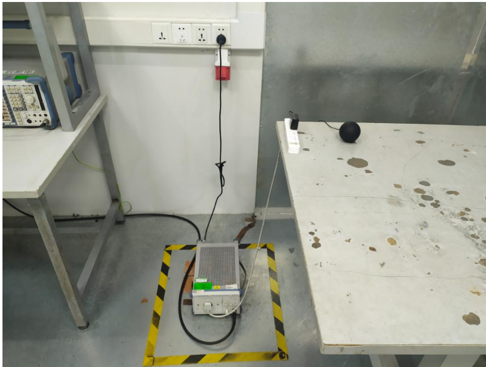
FCC ID: 2AWP6-ODDBALL Photo of Power Line Conducted Emission Test
