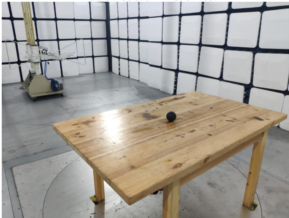
Photo of Radiation Emission Test
