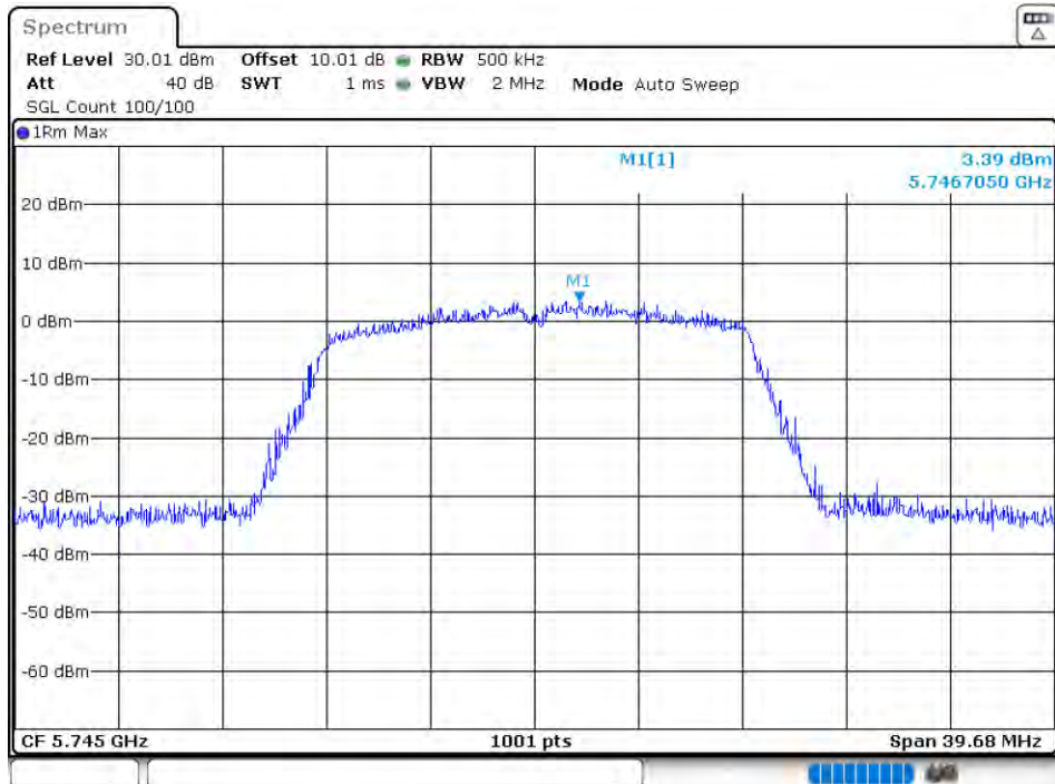
PSD NVNT 802.11a 5745MHz Ant1
