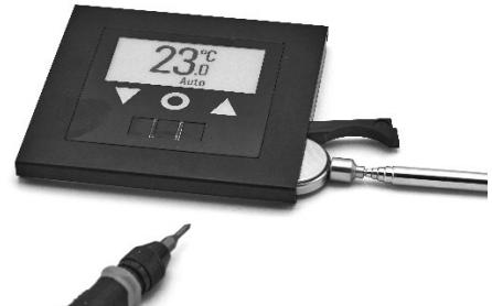
4. Insert the battery with the positive (+) terminal facing the wall.
