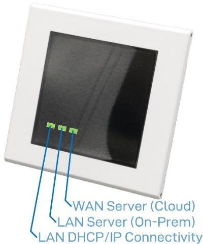
The ER513 features three LEDs on its front side. The LED on the left shows the basic Ethernet connectivity status, such as when the device has a valid IP address. If the LED blinks slowly, the device does not have a valid IP configuration (IP address, netmask). When the blinking turns fast, the device has obtained successfully an IP configuration. If the configuration is not static, it is normally assigned by a DHCP server serving the LAN.
