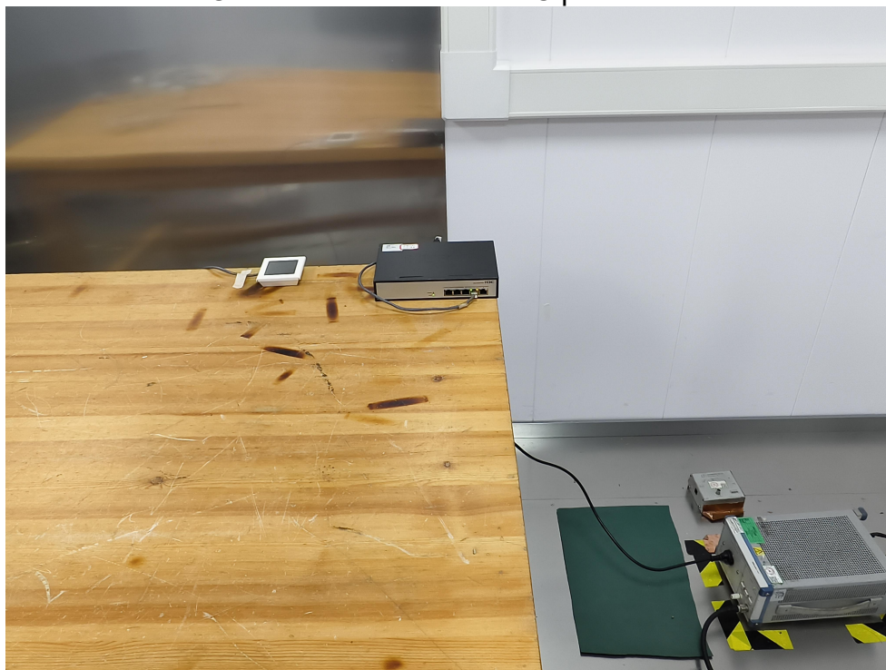
Conducted Emission at AC power line
