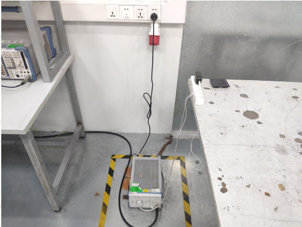
Photo of Power Line Conducted Emission Test
