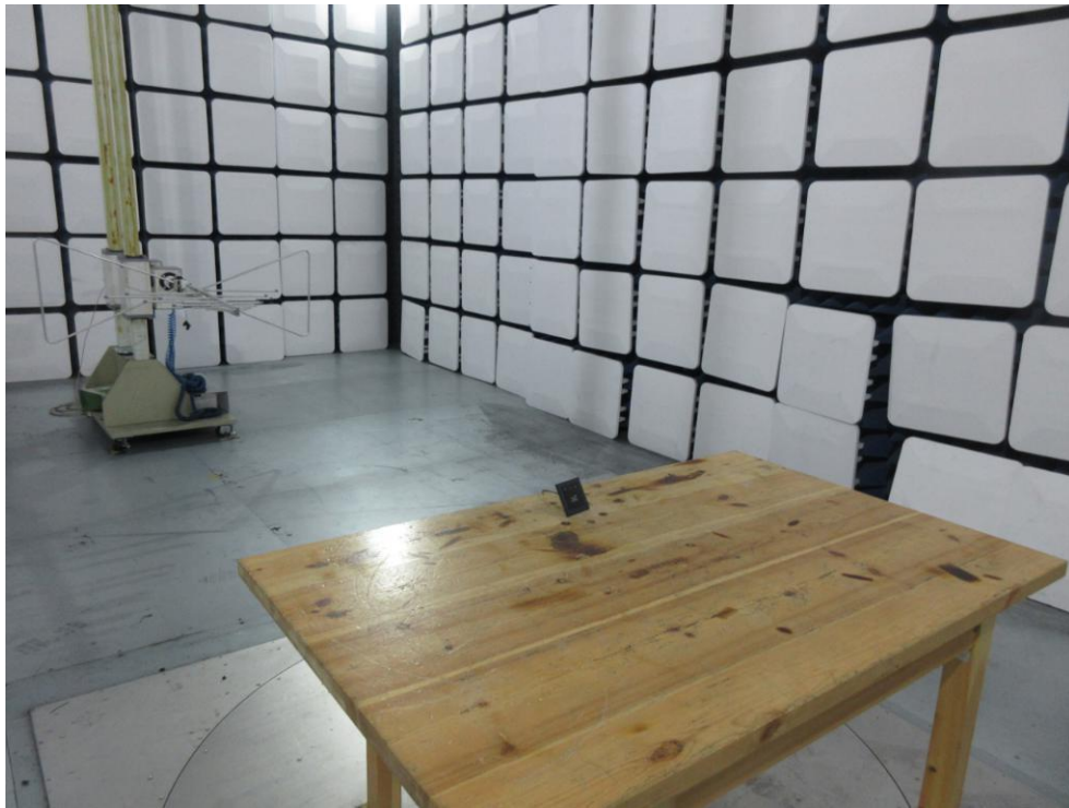
FCC ID: : 2AWOQ-003001C513 Photo of Radiation Emission Test
