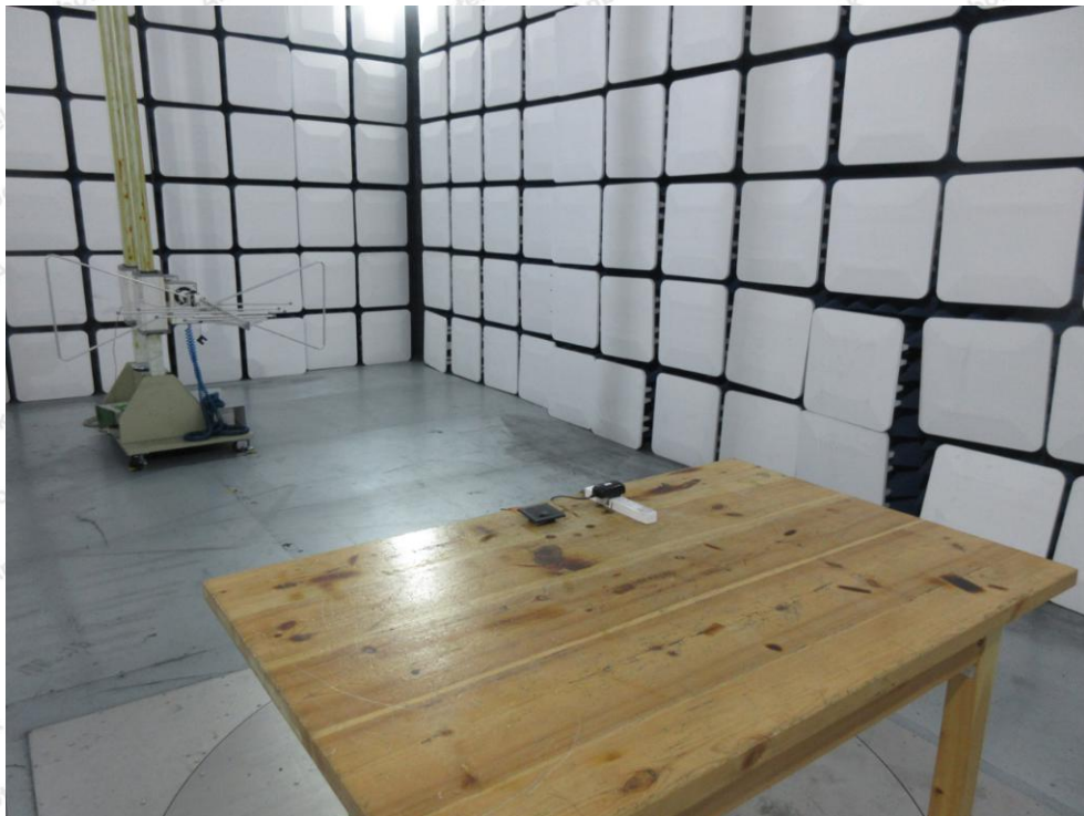
Photo of Radiation Emission Test
