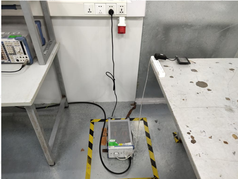
Photo of Power Line Conducted Emission Test
