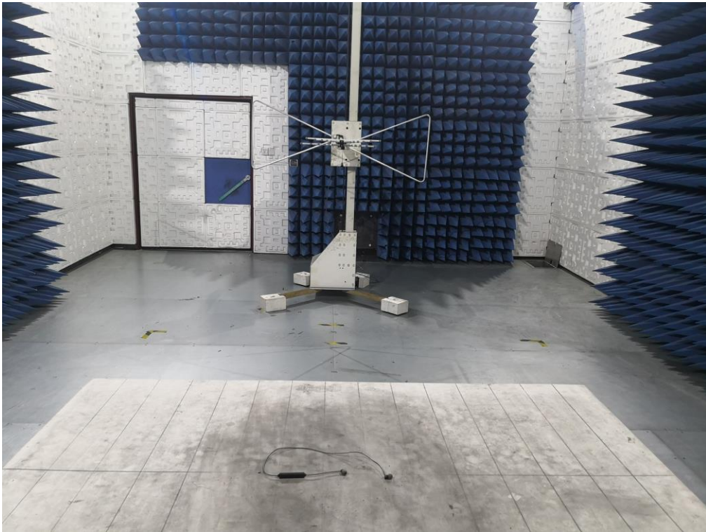
RADIATED EMISSION TEST SETUP ABOVE 1GHZ
