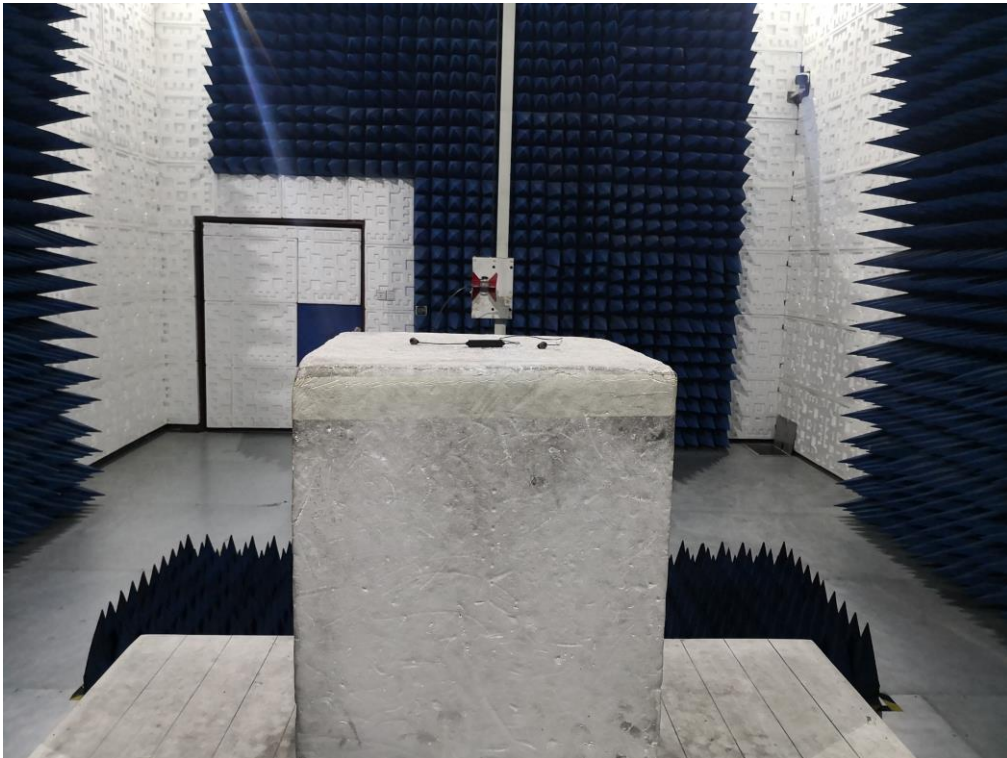
RADIATED EMISSION TEST SETUP ABOVE 1GHZ
