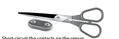
Short-circuit the contacts on the sensor using a metal object such as scissors.
