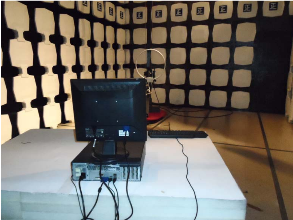
Measurement of Radiated Emission Test Set Up
