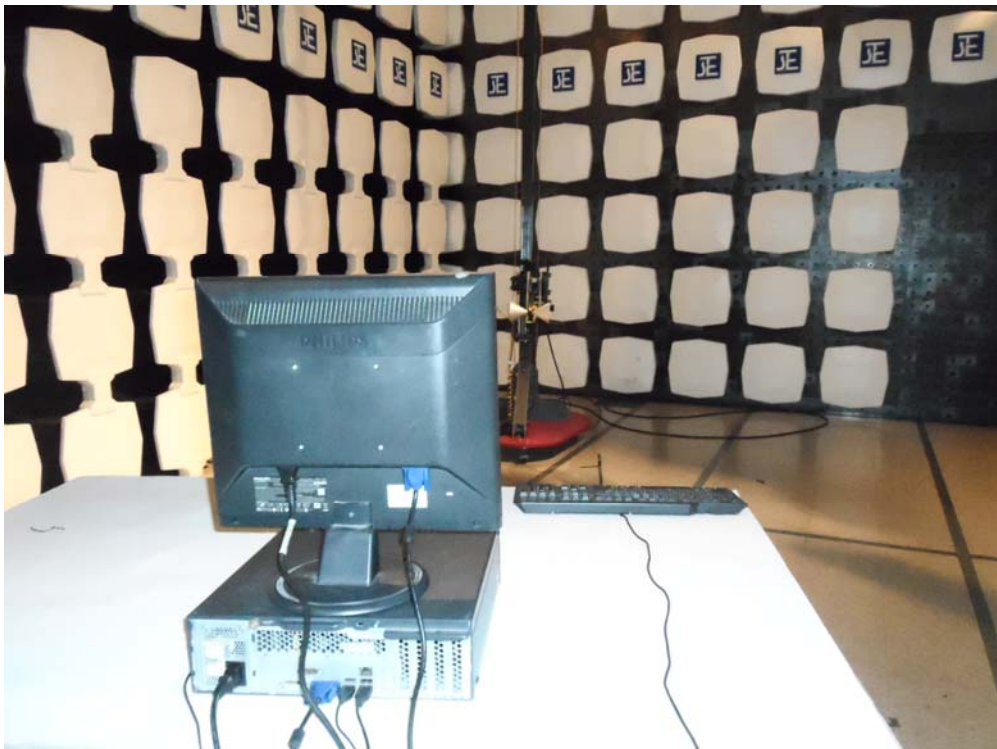
Measurement of Radiated Emission Test Set Up
