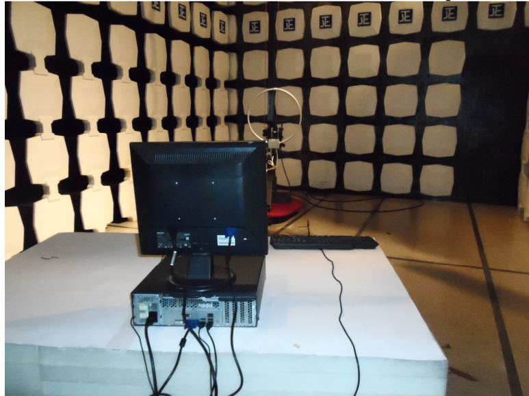
Measurement of Radiated Emission Test Set Up
