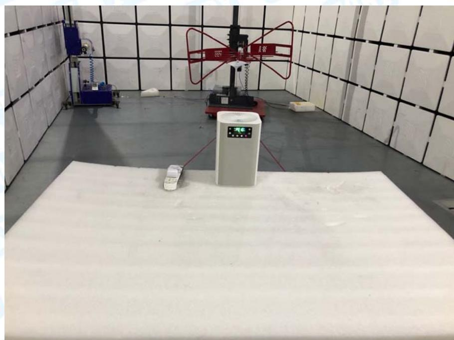
**Photo of Setup for Conducted Emission**
