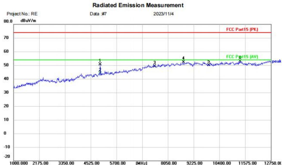
Site: Limit: FCC Part15 (PK) EUT: Bluetooth module M/N: PTR5638 Mode: BLE-1M TX-2480 Note: Polarization: **Vertical** Power: Temperature: (C) Humidity: %RH
