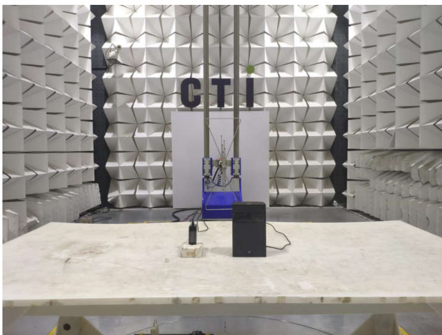
Radiated spurious emission Test Setup-2 (Below 1GHz)
