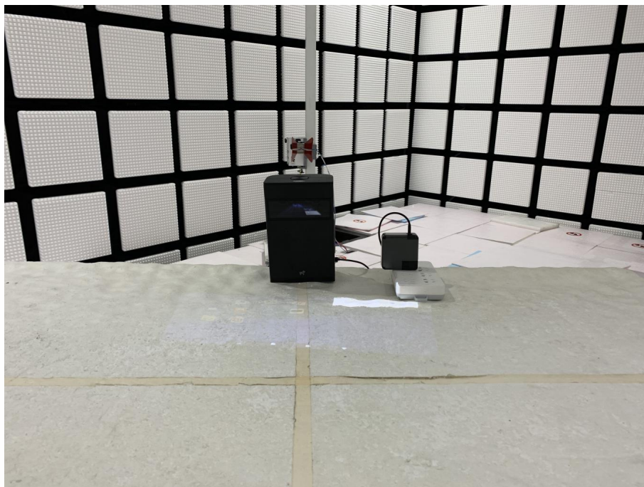
Radiated spurious emission Test Setup-3(Above 1GHz)
