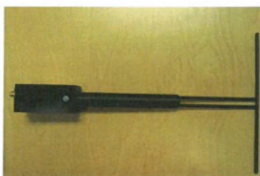
Figure 1 – MVG COMOSAR Validation Dipole
