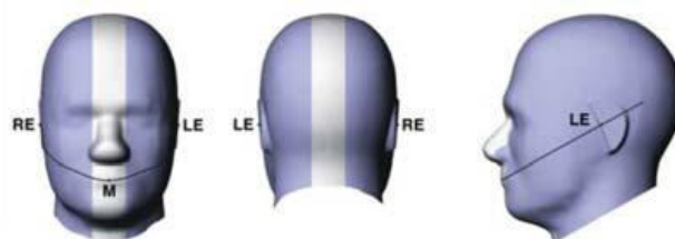
Figure 6.2 Front, back and side view of SAM
