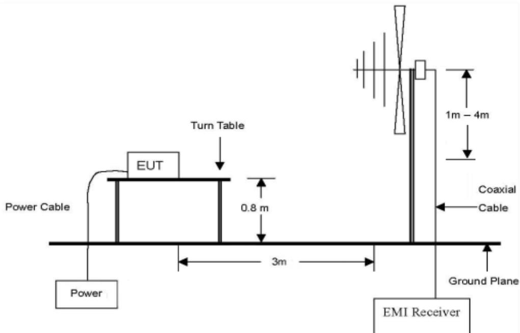
The diagram below shows the test setup that is utilized to make the measurements for emission. The spurious emissions were investigated from 1 GHz to the 10<sup>th</sup> harmonic of the highest fundamental frequency or 40 GHz, whichever is lower.
