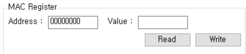
The interface for the MAC Register is a rectangular box with a light gray border. At the top left, it says "MAC Register". Inside, there are two input fields: "Address : ". To its right is "Value : ". Below these fields are two buttons: "Read" (gray background, white text) and "Write" (gray background, white text). The entire interface is set against a white background with a vertical gray line on the right side.
