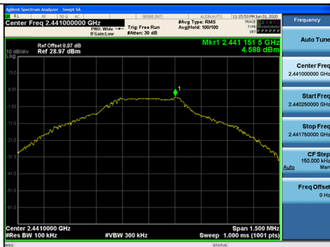
GFSK on Channel 39
