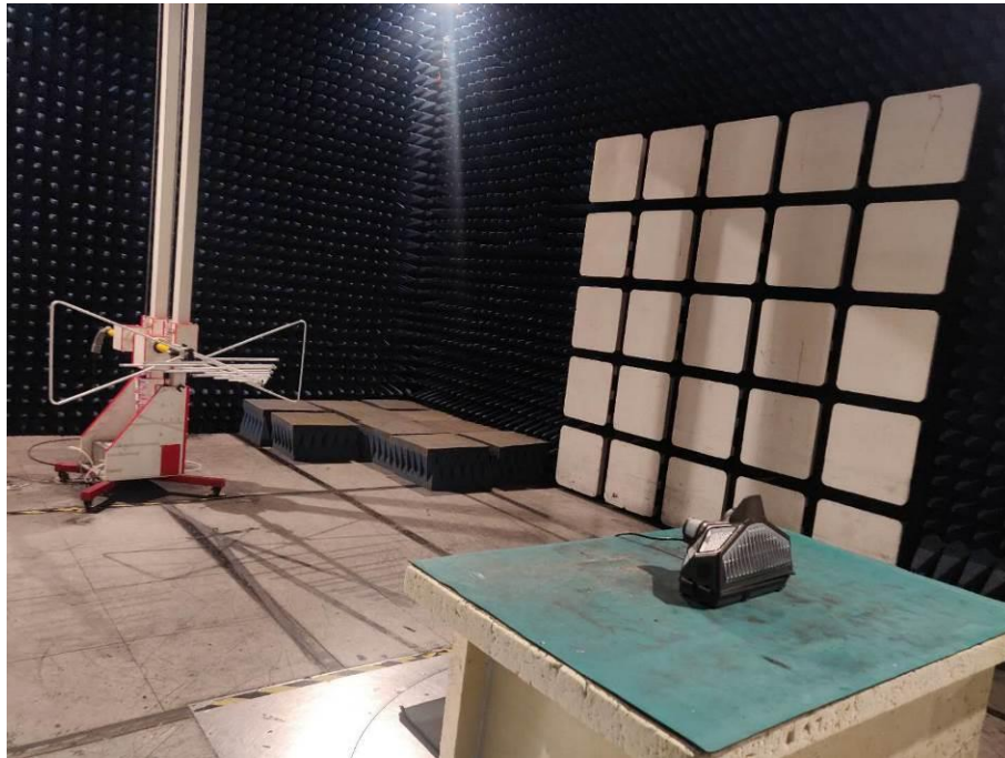
Spurious Emission Test Setup (Below 1GHz)
