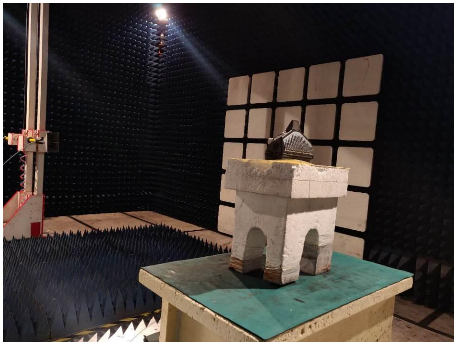
Spurious Emission Test Setup (Above 1GHz)
