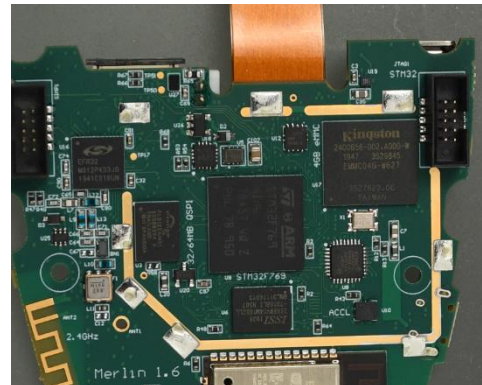
Main Board with Shield Removed
