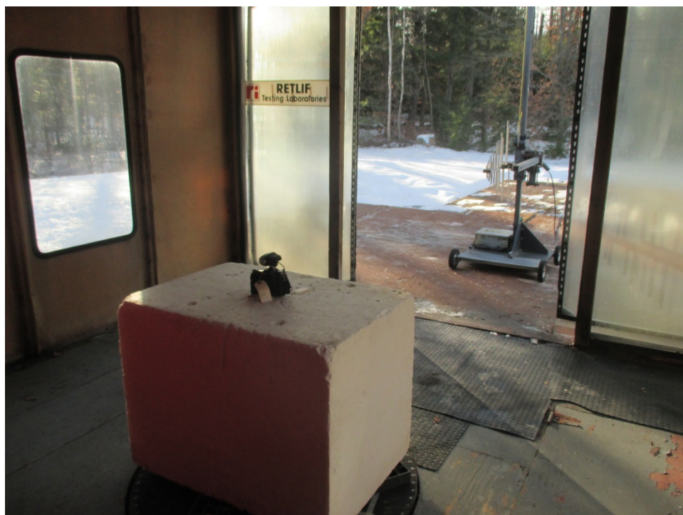
Vertical Antenna Polarization, Below 1 GHz
