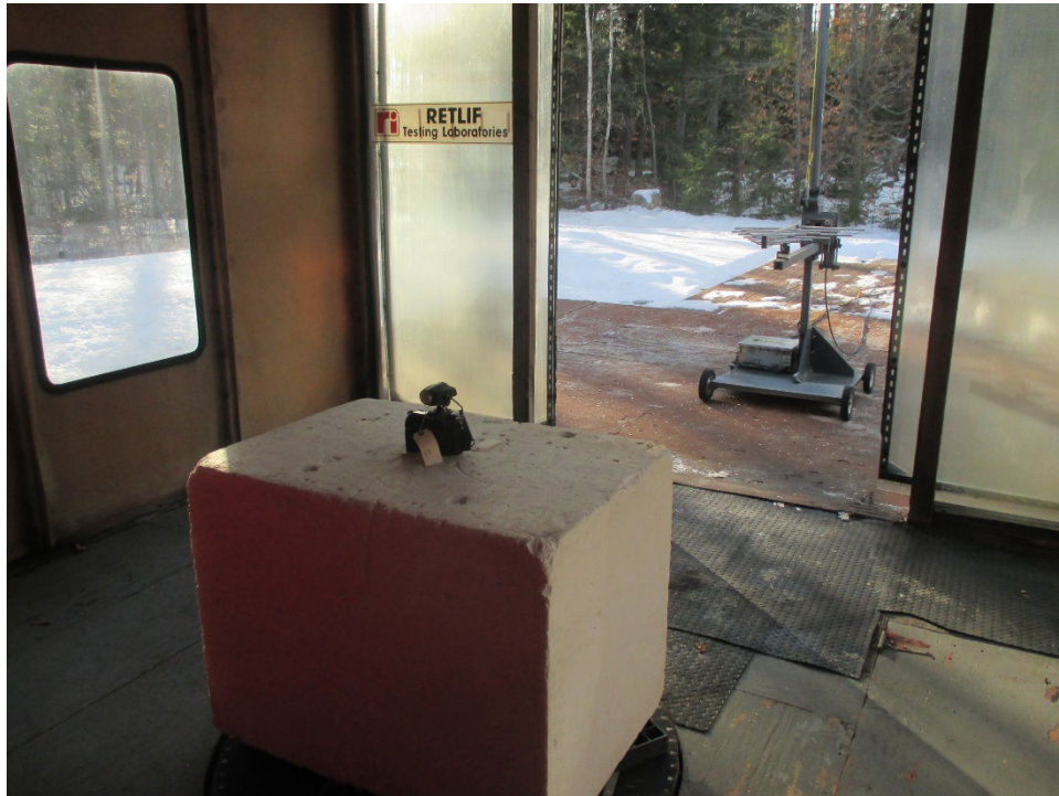
Horizontal Antenna Polarization, 30 to 200 MHz
