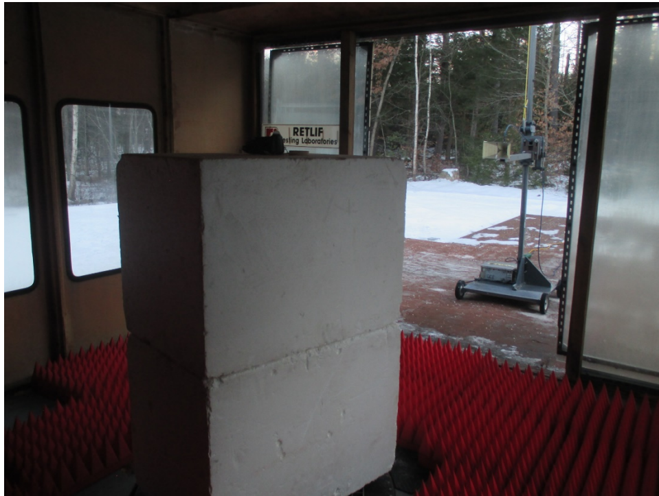
Horizontal Antenna Polarization, 200 MHz to 1 GHz
