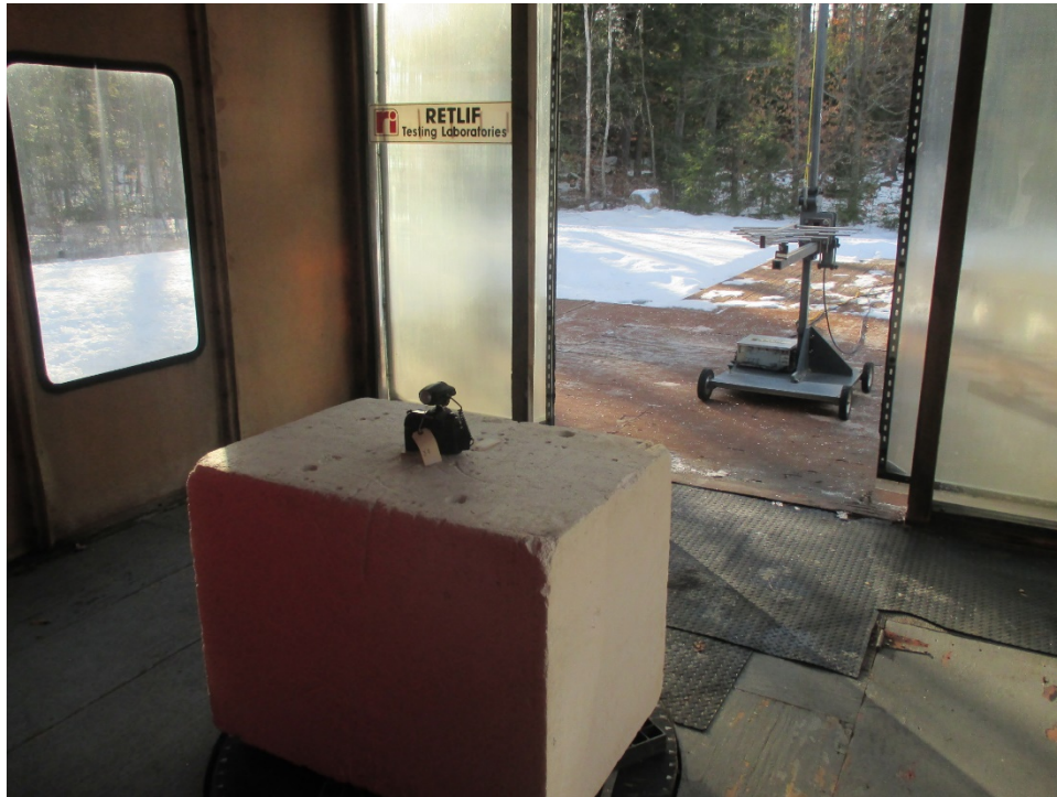
Horizontal Antenna Polarization, 200 MHz to 1 GHz
