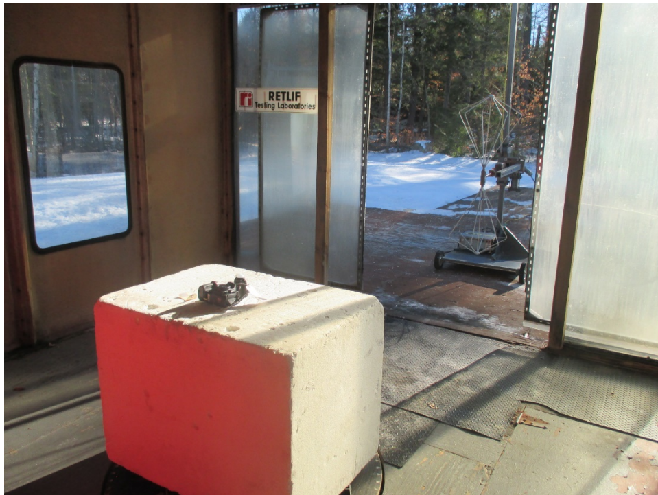
Vertical Antenna Polarization, 30 to 200 MHz
