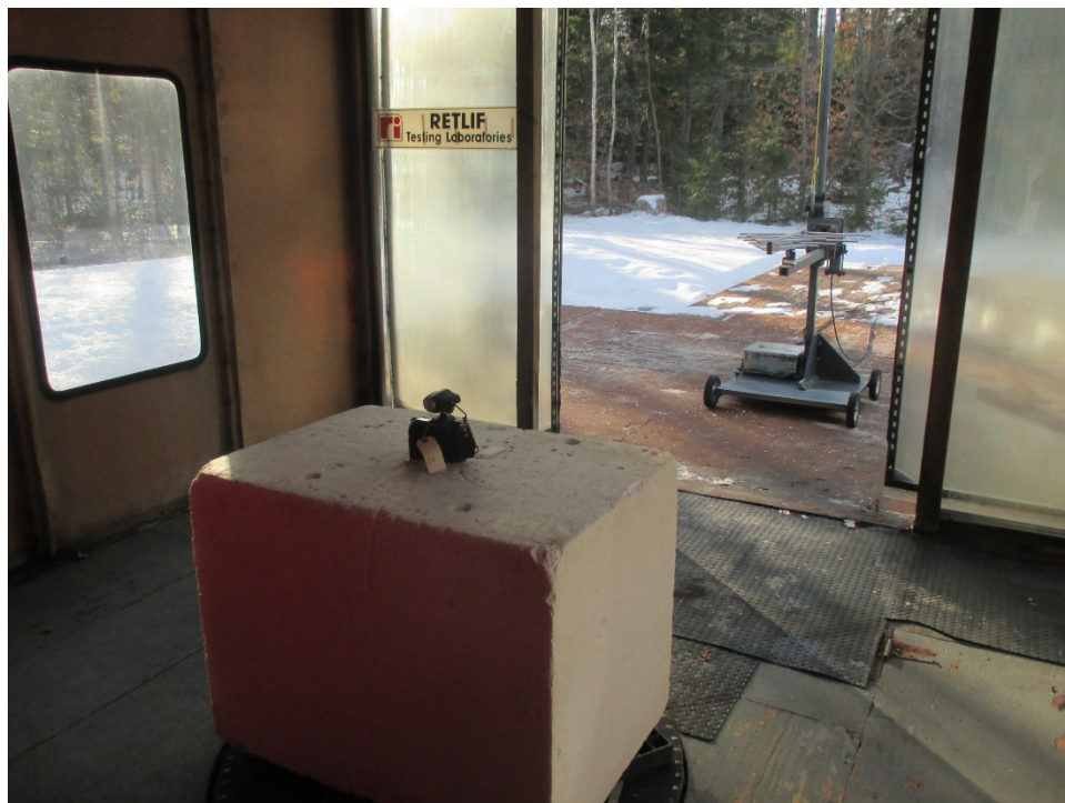
Horizontal Antenna Polarization, Below 1 GHz
