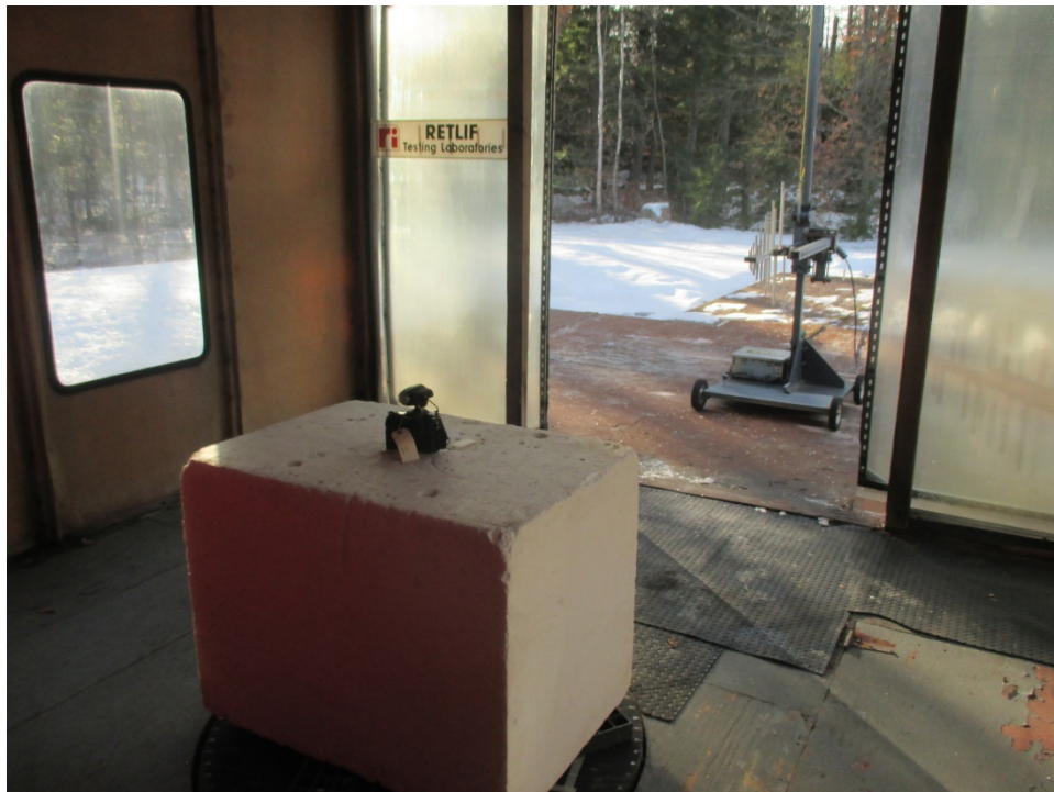
Vertical Antenna Polarization, 30 to 200 MHz
